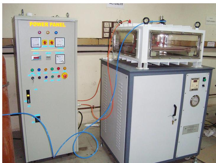
Figure A.5.1.2. (RIGHT) Photograph of the atmospheric pressure plasma processing system
