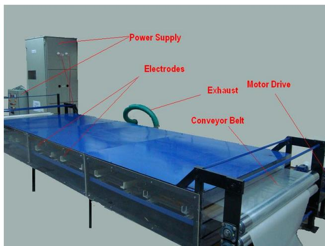
Figure A.5.3.1. Industrial scale non-thermal atmospheric pressure air plasma processing system
