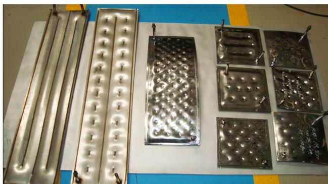
Figure A.2.3.1 Prototype Cryopanel developed for Cryosorption Cryopump Project.
