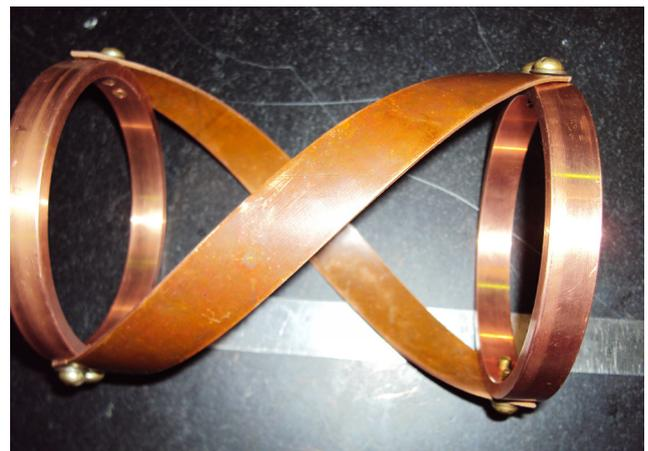
Figure A.3.6.2 Helicon antenna  $M=+1$  having 180mm length and 108mm internal diameter
