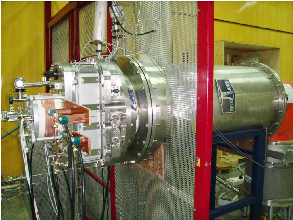
Figure A.2.5.2 : RF ion source experimental set up in the negative ion laboratory
