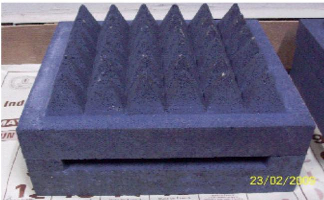
*Figure A.1.2.3.2 Black body radiator for calibration*
