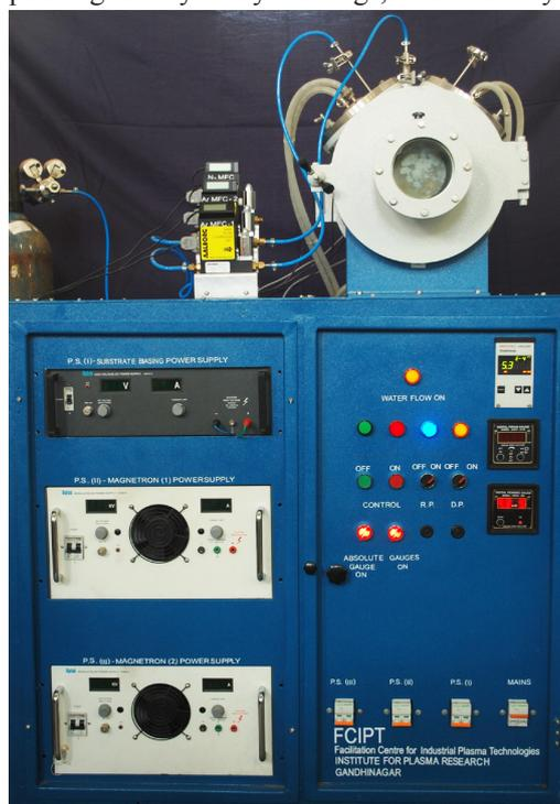
Figure A.5.1.1 : (LEFT) Photograph of the twin magnetron system
