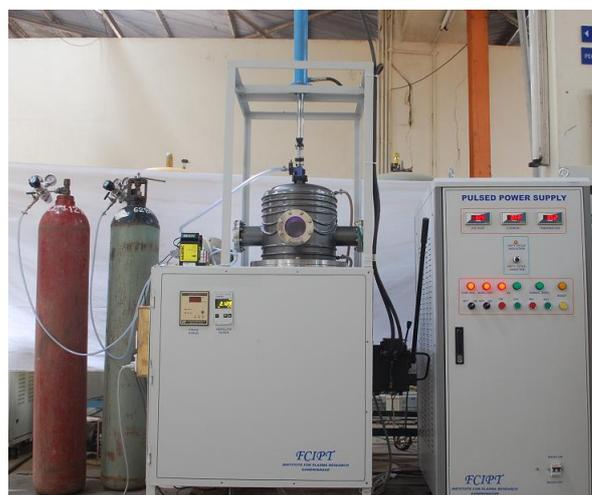
Figure A.5.3.2. Lab scale plasma glow-discharge system, developed at FCIPT for MG University, Kerala
