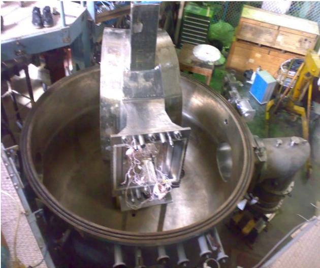
Figure A.1.2.2.7 A vessel module getting ready for the baking in a dedicated baking facility
